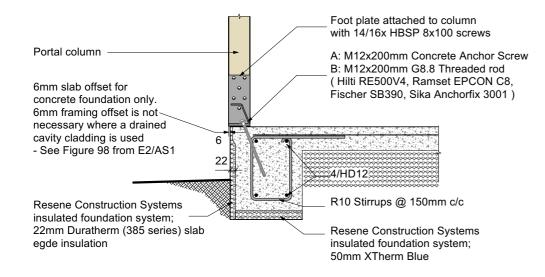
Note: Refer to D1104, D1113, D1114 for slab edge installations
