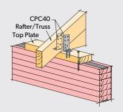
Avoid drilling through or damaging the steel bar for fixings and take care to prevent the steel plate from damaging the screw threads.
