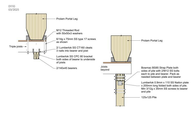
As per NZS:3604 for any builds in Zone D, subfloor fixings will need to be stainless steel or denzo taped.
