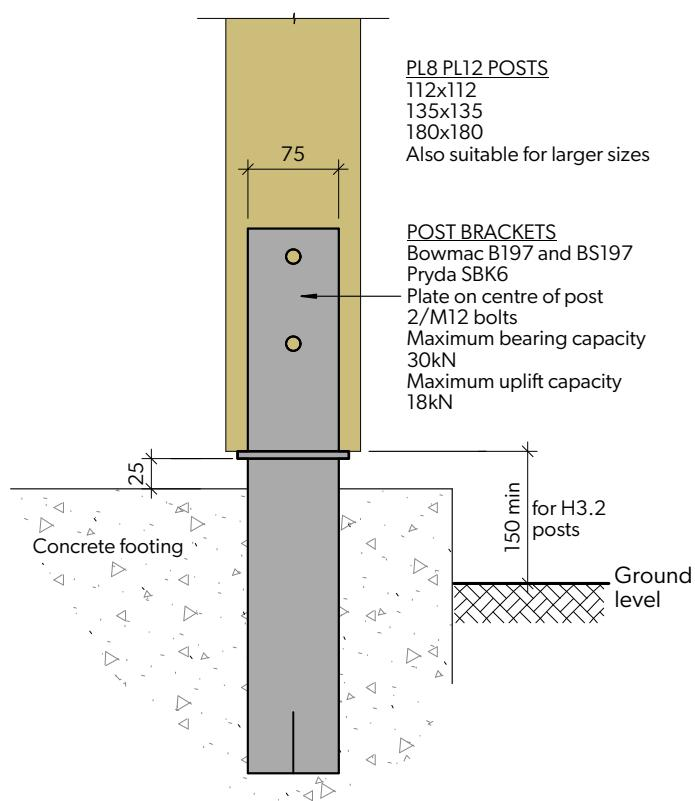
Note: H5 treated posts may be seated on the concrete and be closer than 150mm or embedded into the ground
